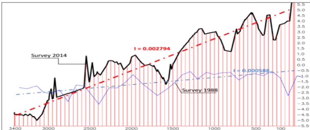
Figure4: Longitudinal profile of downstream Jeneberang Rubber Dam, based on topographic survey 1988 and 2014
